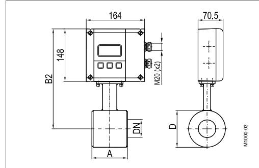
Thanks to its very short lay length, the detector type III is often the right alternative to a lot of applications. Delivered with a PTFE liner, the detector type III has a standard nominal pressure of PN 40.
