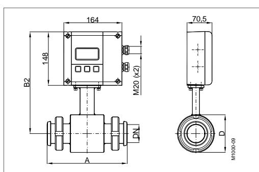
The sanitary detector was developed for the flow measurement of liquid food. This model is available with Tri-Clamp®, DIN 11851, ISO 2852 process connections and also with any special connections (customer specifications). The sanitary detector is delivered in a stainless steel housing and with PTFE lining.
