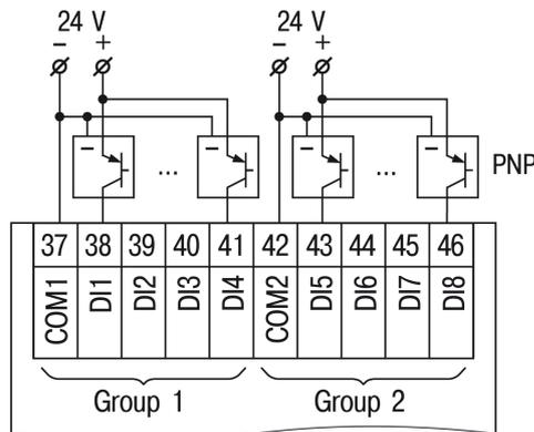
Fig. 5.4 3-wire sensors with PNP transistor outputs
