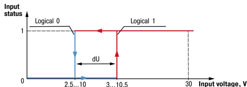
Fig. 4.3 Digital mode of an analog input
