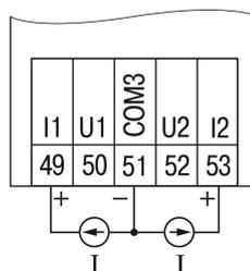
Fig. 5.5 Current signal (4-20 mA)
