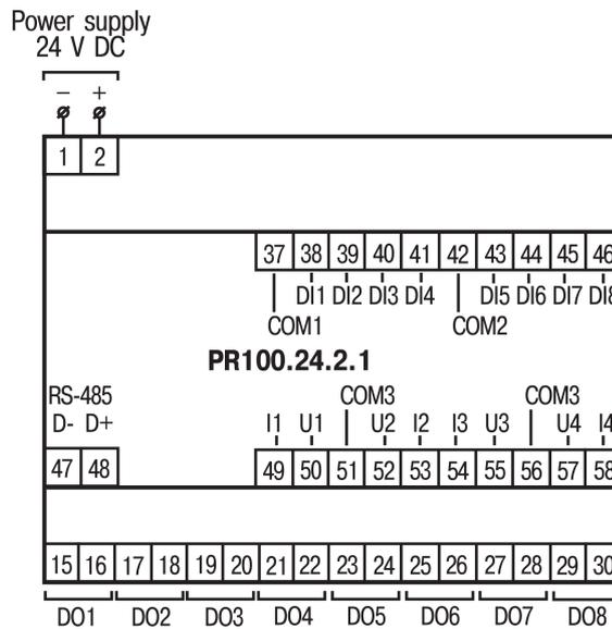
Fig. 5.2 Terminal block layout
