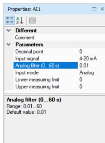
Fig. 4.2 Property Box for analog input
