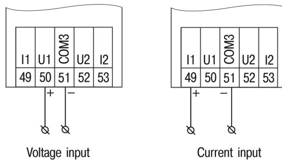
Fig. B.2 Connection of the reference signal source to an input
