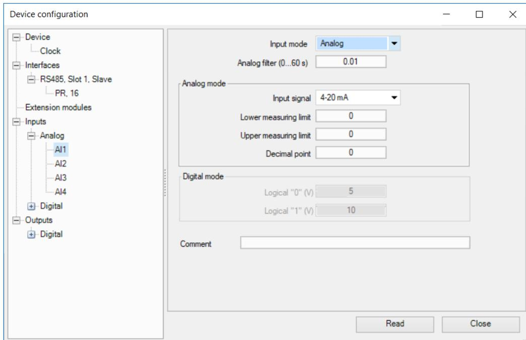
Fig. 4.1 Analog input configuration
