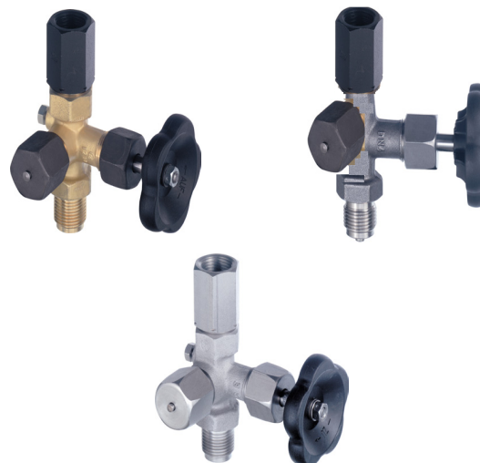
Valve with isolating test connection per DIN 16 271, LH/RH adjusting nut/Male G 1/2, with test connection M 20 x 1.5, PN 400
