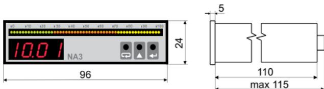
**Fig. 2. Meter overall dimension and fixing way.**
