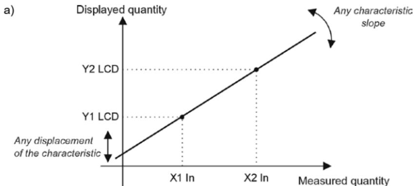
Value  $I_{H1}$  on the meter input  $\Rightarrow$   $d_{Y1}$  on the display.
