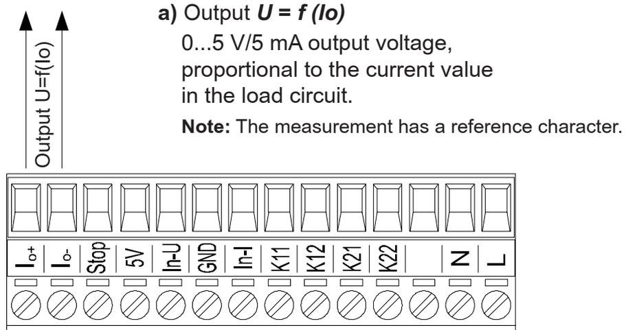
Fig.7. Analog outputs.
