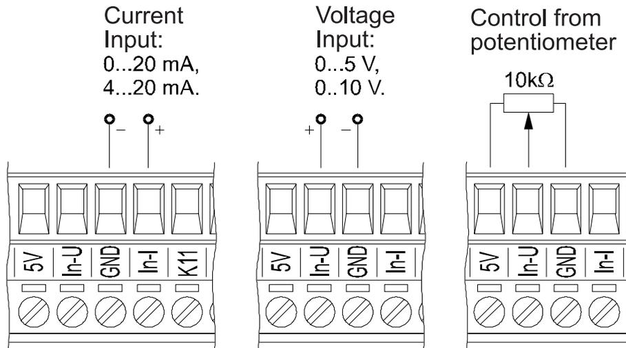
Fig.5. Connection of control signals.
