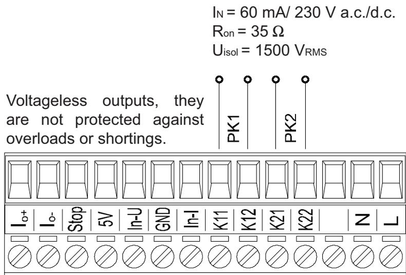
Fig. 8. Relay outputs.
