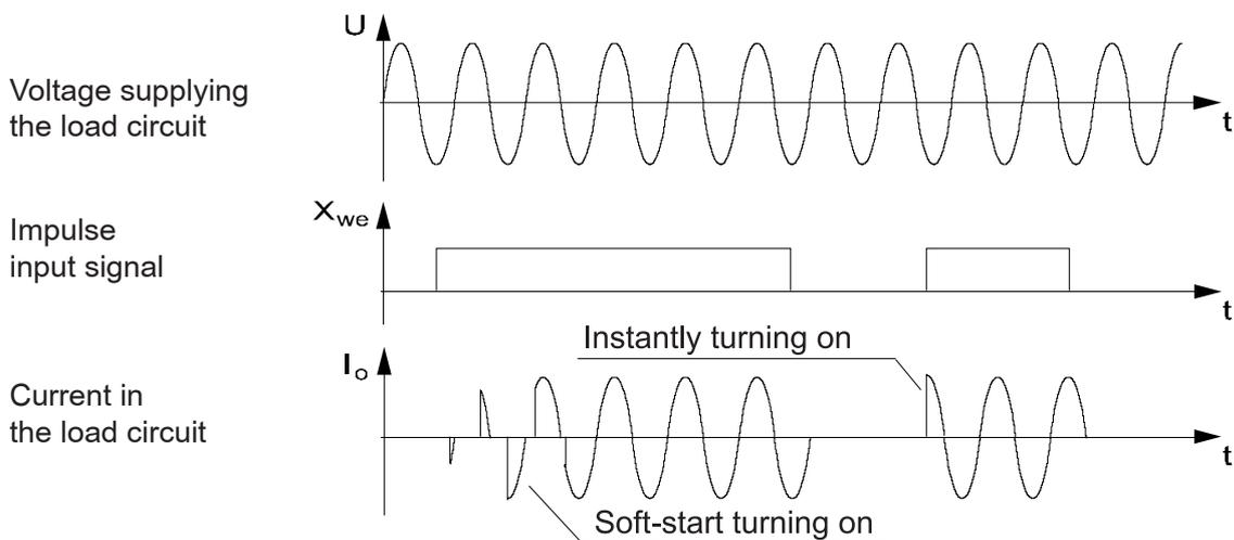
Fig.10. Control of on-off type, runs of occurring signals in relation to the neutral wire - resistance load.
