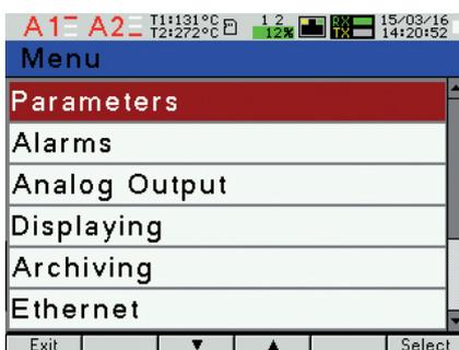
easy to use and intuitive menu; information bar with status of: phase sequence, alarm outputs, temperature measurements\*, archiving and memory\*, Ethernet\* and RS-485 interfaces, time and date
