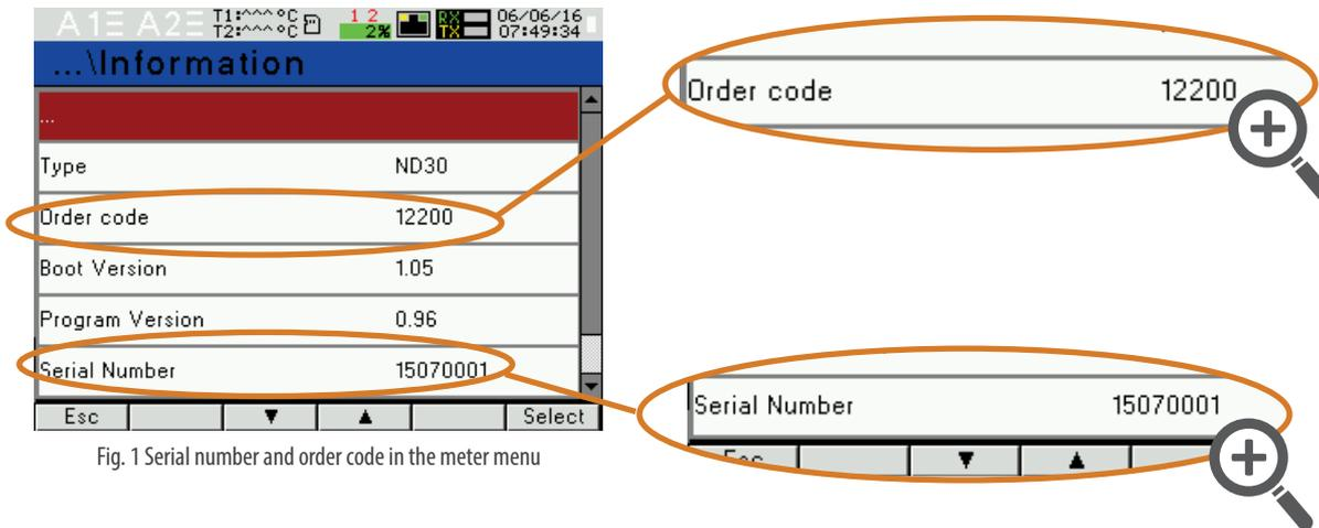
Fig. 1 Serial number and order code in the meter menu
