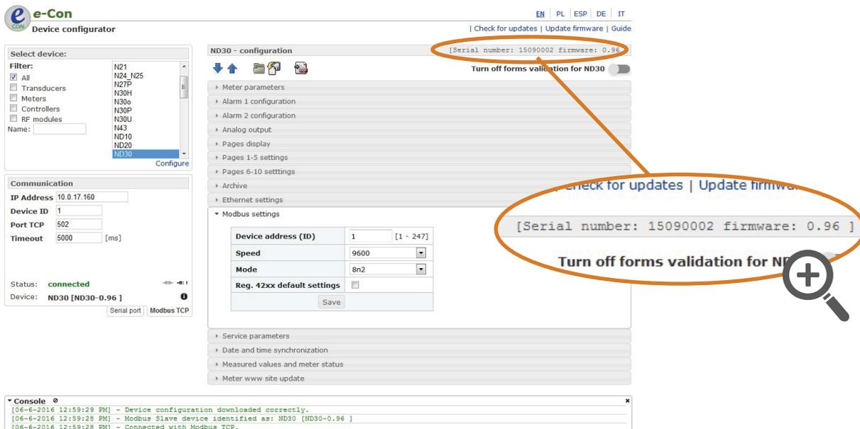
Fig. 2 Serial number in the eCon software bar
