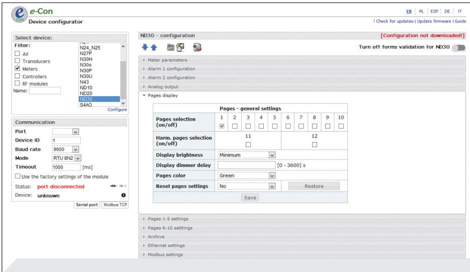
ability to configure and update ND30IoT, ND30 with free eCon software (via RS-485 or Ethernet\* interface)
