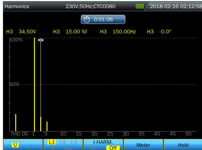
The Bar Graph display shows the percentage contribution of each of the components related to the fundamental or full signal. A signal without distortion should show a 1<sup>st</sup> harmonic at 100% while the others are at 0: in practice this will not occur because there always is a certain amount of harmonics resulting in distortion.
