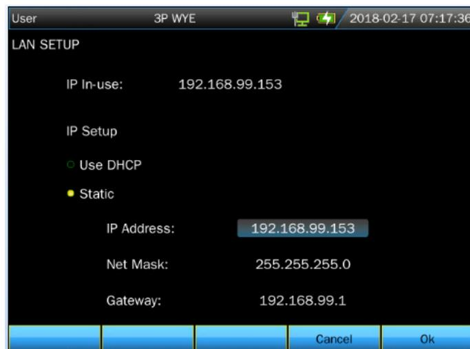
Connect the Analyzer with PC by one piece of net cable, set IP address of Analyzer and PC to different, but should be in the same network segment. For example: IP address in PC is 192.168.1.XXX, while IP address in the Analyzer also should be 192.168.1.XXX accordingly.
