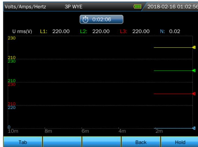
The trend records the data measured in the latest ten minute, then the curve formed from the right side. Reading in the header is correspond to the latest values formed in the right side.
