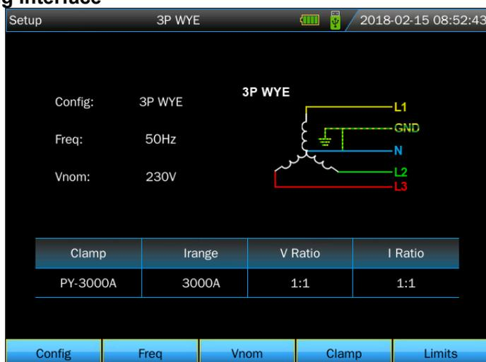
After power on, current setting will be displayed on the top of the screen. Check if the Date and Time of the system clock are correct. Also the wiring configuration must match the configuration of the power system to be checked. The **【SETUP】** key accesses menus to view and change Analyzer settings.
