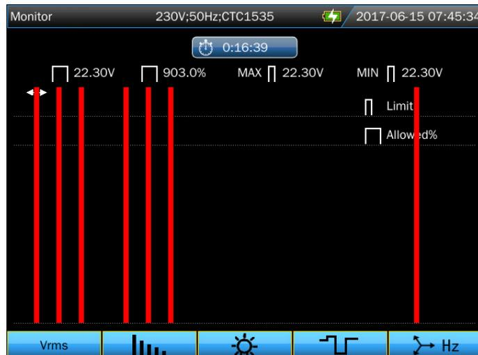
Power Quality Monitoring is reached via the **【MONITOR】** key, and Immediate or Timed start is settable. With the direction keys you can position the Cursor on a particular Bar Graph. Measuring data belonging to the bar is shown in the screen header.
