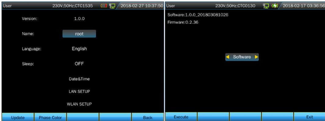
There are tree types of update file including Software, Firmware and System. Select you wanted files to update, the Analyzer will give prompt after finishing update, then plug out the U disk, power off the Analyzer then power on to complete the update.
