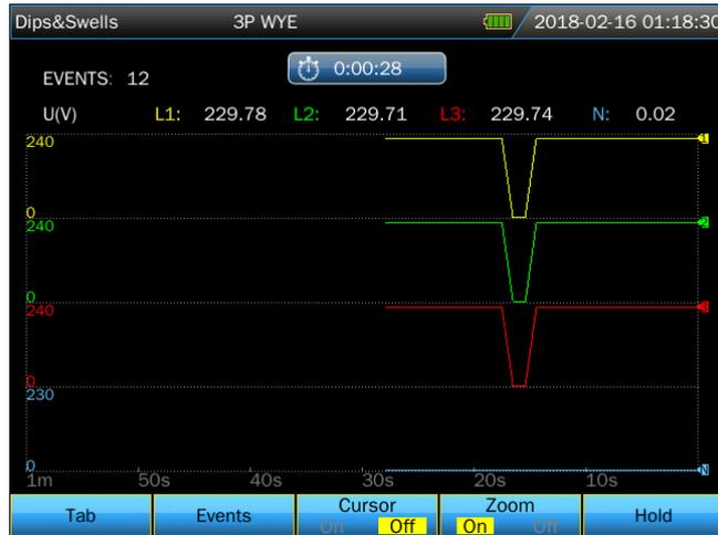
Both voltage and current are recorded to help user to observe causation of causing deviation.
