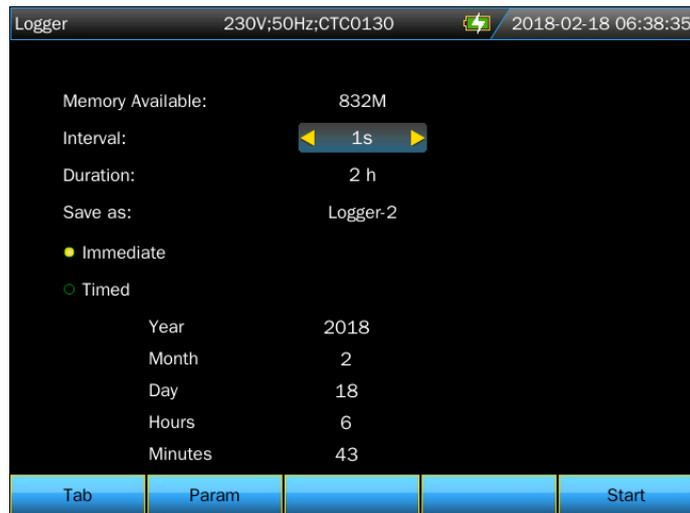
Here user can check remaining storage space, choose the needed logger parameters, set record interval, duration time and name of stored file. Then press **【F5】** to start.
