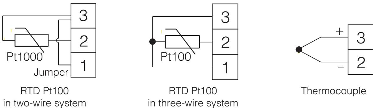
Fig. 4. Connection of input signals
