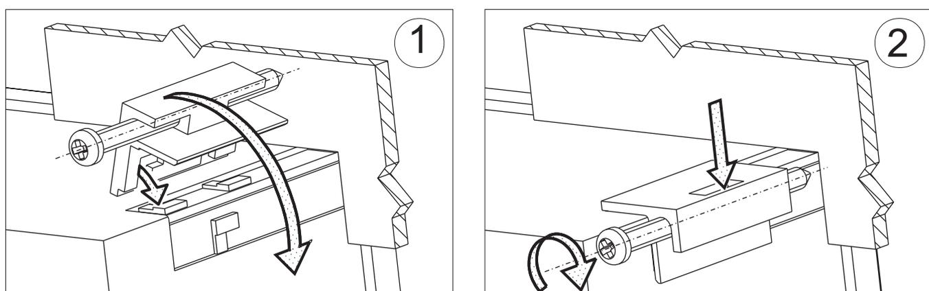
*Fig. 1. Controller fixing in the panel.*
