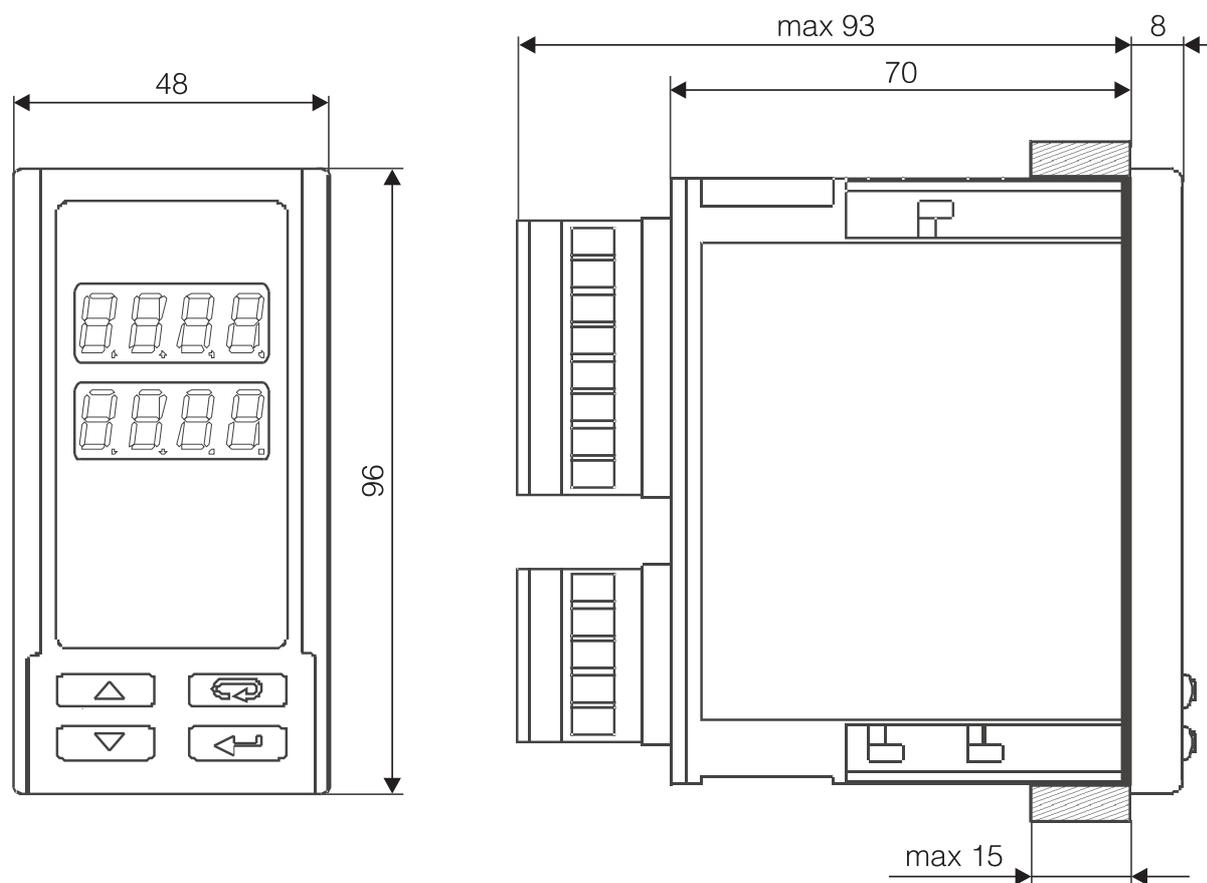
*Fig. 2. Controller overall dimensions*
