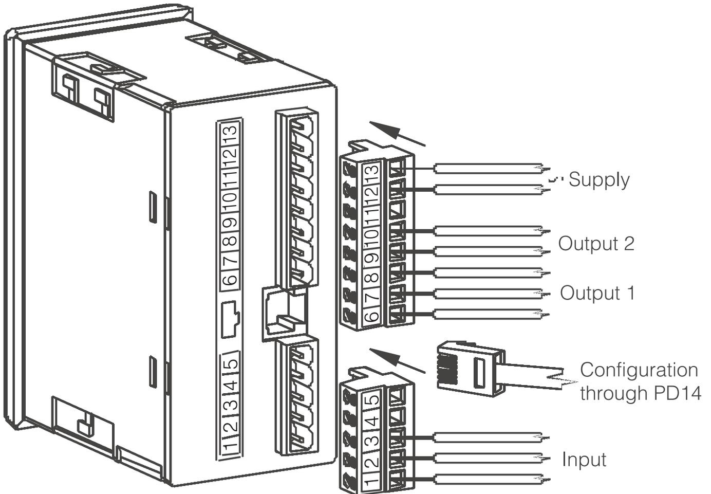
Fig. 3. View of controller connection strips
