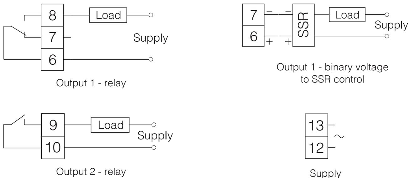
*Fig. 5. Supply and load circuit connection*
