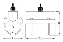
**NZ, WZ, HZ, LZ, YZ** Pipes Larger than 2 in. (50 mm)
