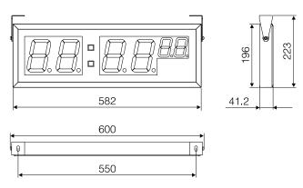
Fig. 1 View of the DLZ clock and overall dimensions
